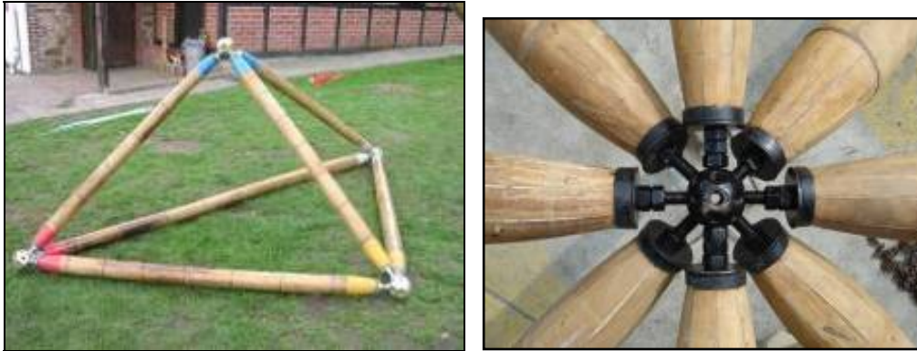
Photo 21, 22: Very powerful for axial bolts are conical bambú joints and MERO sphere.
