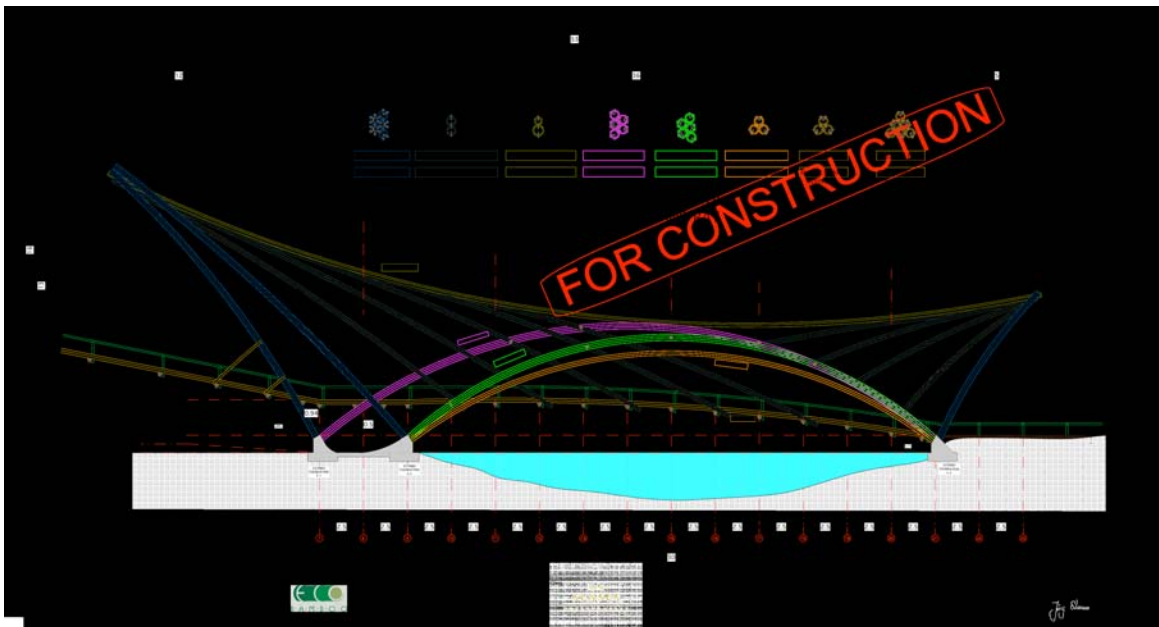
Construction Drawing of the 30m bamboo Bridge at Soneva Kiri Resort, Koh Kood, Thailand. Shpwn are the “double footing” on the left, and lettered are the “Ray beams” A-L. Above the construction details shows the coupled bamboo elements- Triangular 3-pack, 5-pack, Triangular 6-pack.
