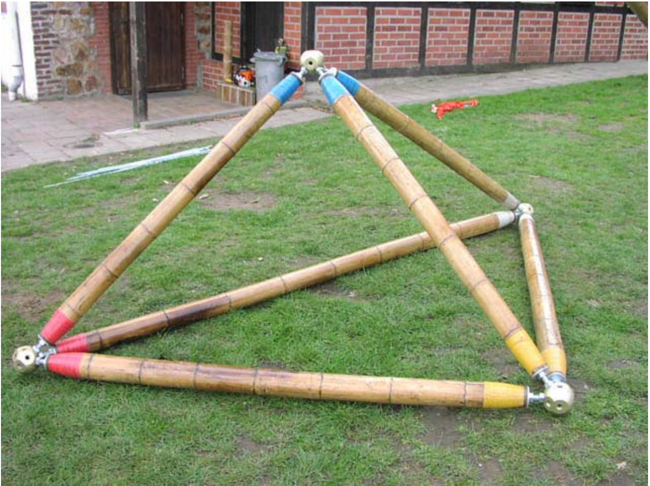
Figure 18 The development of bamboo connection to avoid eccentricity of load transfer with a space frame connector (Courtesy of Evelin Rottke)
