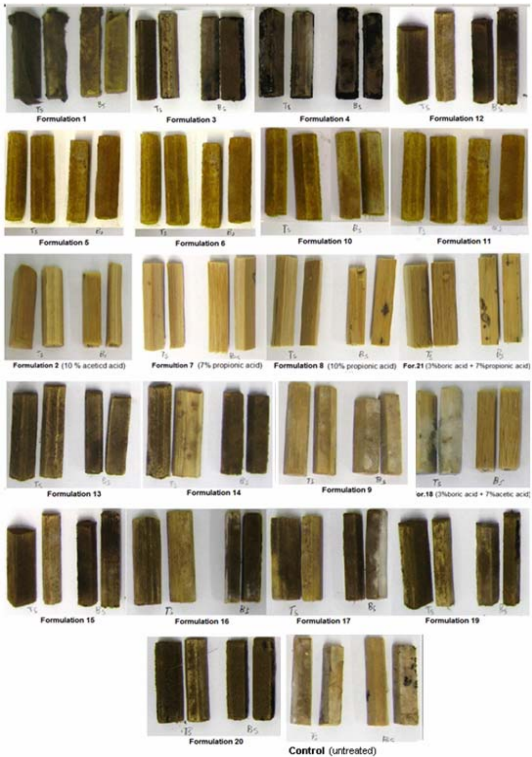
Figure 3. Artificially infected and differently treated bamboo specimens after 8 weeks of incubation
