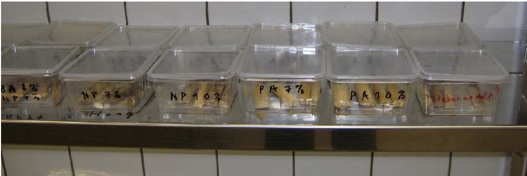
Figure 2. Specimens in plastic basins for mould protection test
