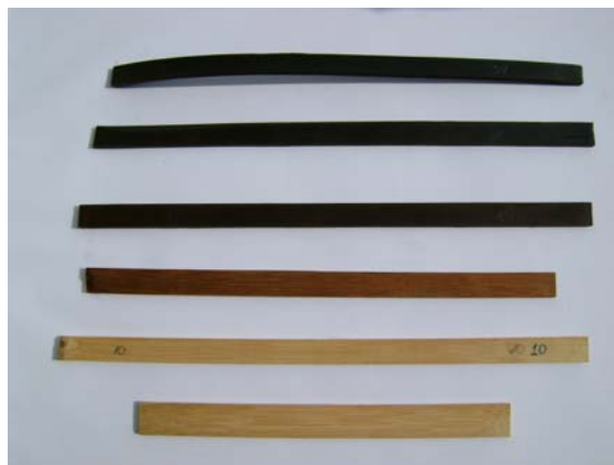
Figure 1 – TTB according to the thermal treatment temperature (air dried – control; 140, 180, 220, 260 and 300 °C (upper)).
