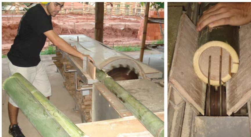
Figure 3 - Transversal cutting and longitudinal cutting.
