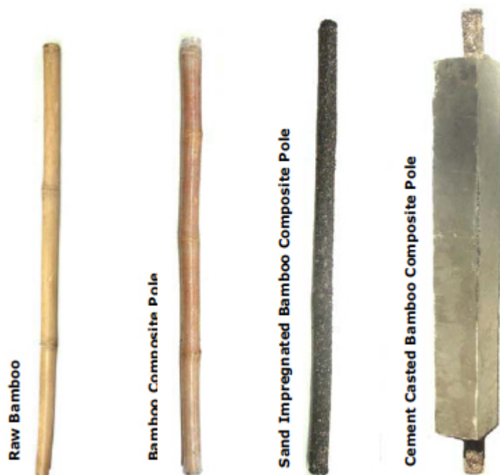
Figure 13 : Making of the Cement Casted Bamboo Composite Pole
