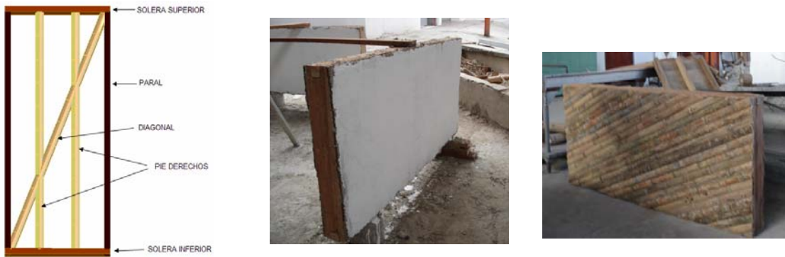
Figure 9. Structure of the guadua board. Board of guadua of bahareque encementado. Board with narrow sheets cover.
