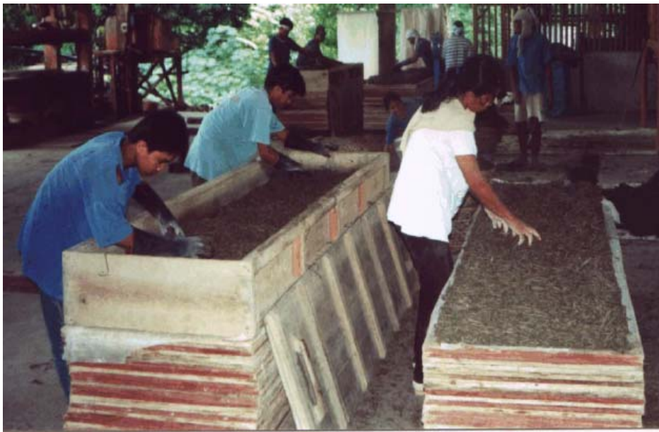
Figure 1. Manual mat-forming of cement-coated wood wool strands in a commercial WWCB plant in the Philippines
